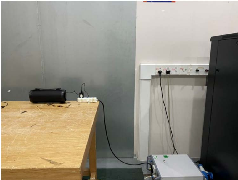
Conducted disturbance at mains terminals Test
